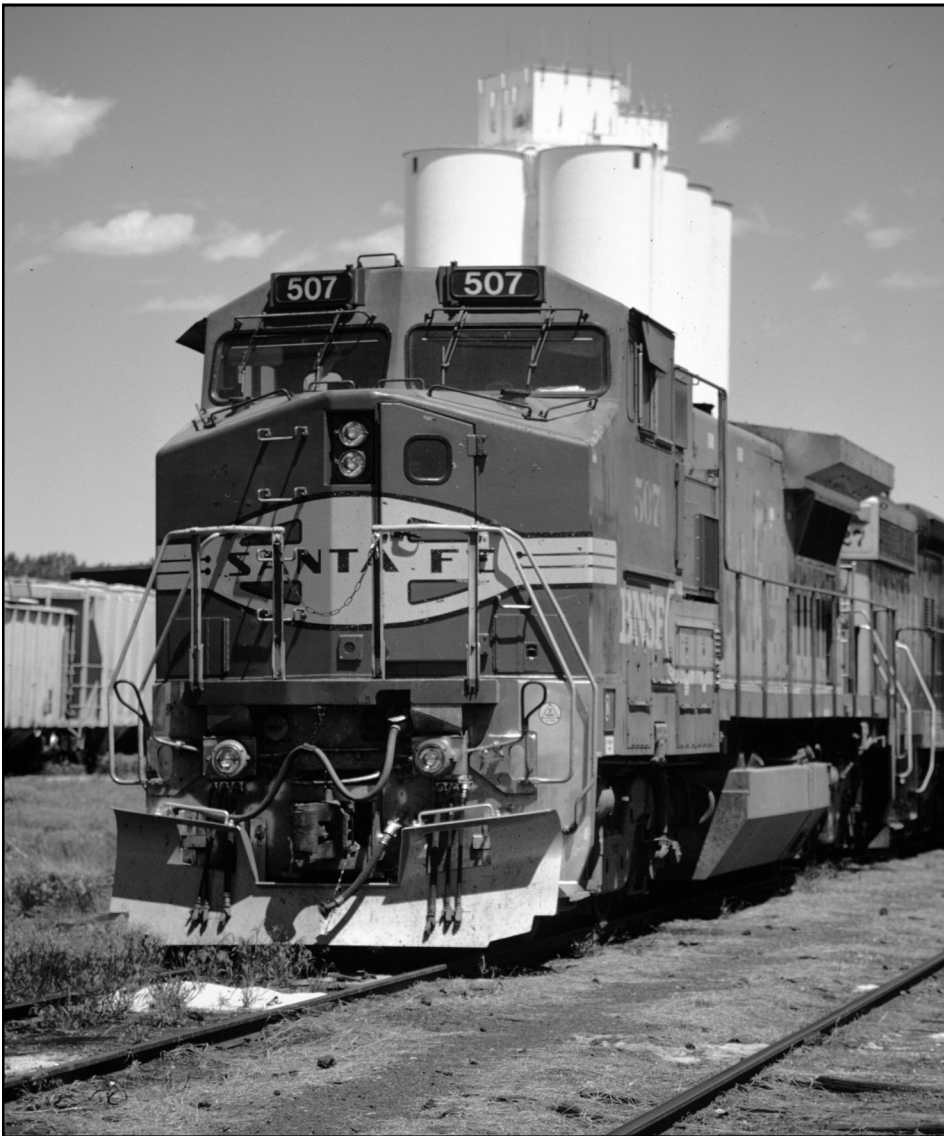
BNSF is having several locomotives repainted by the Omnitrax Shop at Loveland, CO. Several former Santa Fe 500-series (General Electric model 8-40BW) units have been repainted into BNSF's Heritage II scheme. BNSF 507 was at Loveland on 5/24/01 for repainting later that month. – Photo © Chip.
